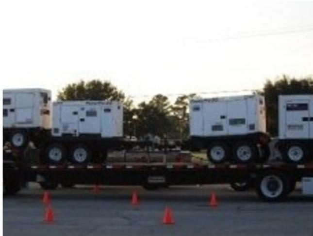
**Generators:** The movement of water for potable purposes and firefighting requires electrical energy, which may not be available in an emergency. Consider backup, alternate, and portable energy sources such as generators.
